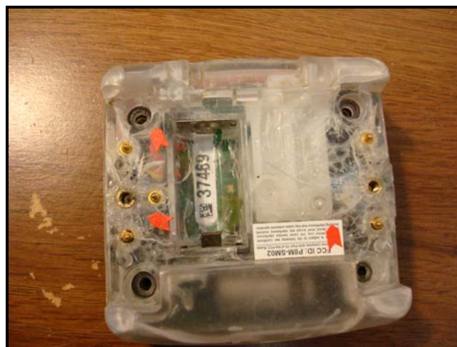
Figure 13: Damage Due to Crushing
