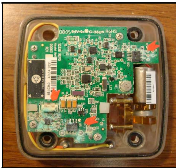
Figure 11: Corrosion Due to Submersion
