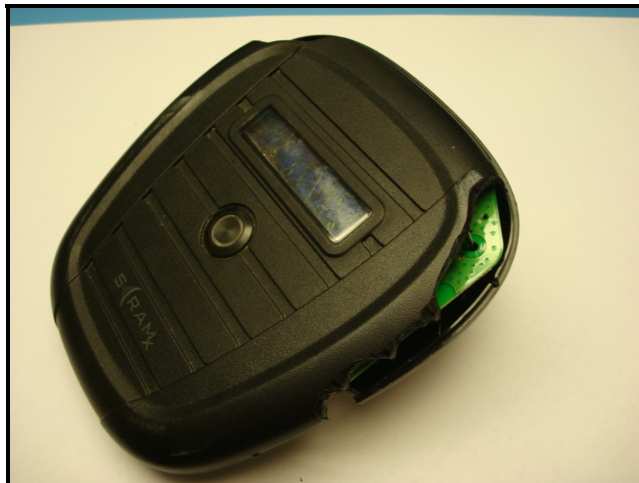
Figure 15: Damage Due to Throwing
