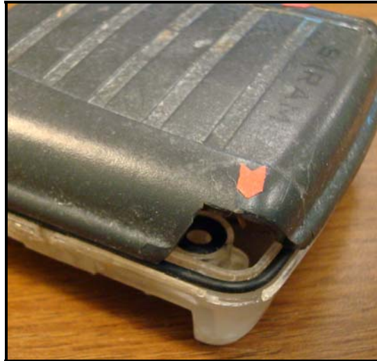
Figure 12: Damage Due to Tampering
