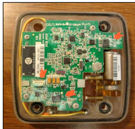
Figure 1: Non-Warranty Repair Example - Corrosion consistent with submersion in water
