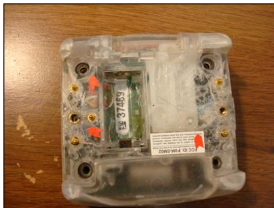
Figure 3: Non-Warranty Repair, Crushed - Bracelet was returned crushed
