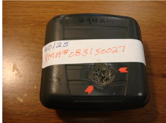
Figure 4: Non-Warranty Repair, Fire Damage Example - Bracelet had a deep burn in the plastic
