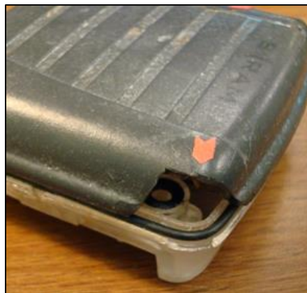
Figure 2: Non-Warranty Repair, Tampered Example – Bracelet was returned after being cut open
